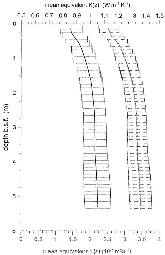
**Figure 9.** (left) mean equivalent thermal conductivity ( $\bar{k}_{eq.}$ ) versus depth  $\pm$  S.D., computed using the thermal resistance method [Bullard, 1939] for increasing sediment thickness on the data shown in Figure 3 and (right) corresponding mean equivalent thermal diffusivity.
