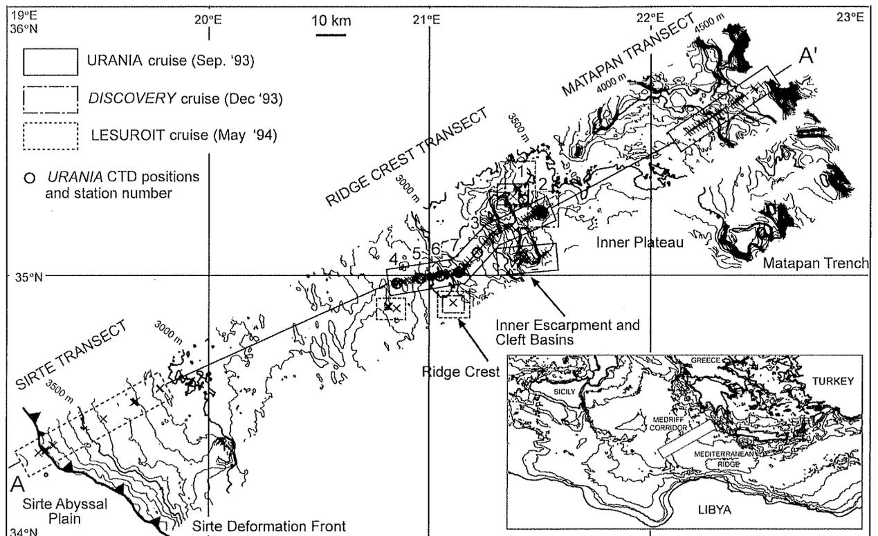
**Figure 1.** Location of the 154 heat flow measurements (crosses) collected during the three MEDRIFF cruises. Multibeam bathymetry is from *L'Atalante* cruise Heralis, 1992. The bathymetric profile A-A' is displayed at various scales, in whole or partly, in Figures 2, 5, 7, 8, and 13. Navigation and positioning was GPS controlled.
