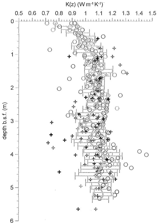
**Figure 3.** Thermal conductivity ( $k$ ) measurements on cores GC-03, PC-04, PC-06, and GC-09 (open circles) and in situ (crosses) from the ridge crest area. Average interval  $k$  every 10 cm and the corresponding standard deviation were computed using a 30 cm moving window.
